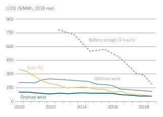
Source: BNEF. Note: The global benchmark is a county-weighted average using the latest annual capacity additions. The storage LCOE is reflective of a utility-scale, lithium-ion battery storage system running at a daily cycle and includes charging costs assumed to be 60% of wholesale base power price in each country.
