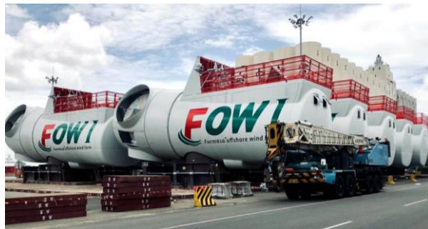
Wind turbine nacelles at Taichung Port ready for installation
